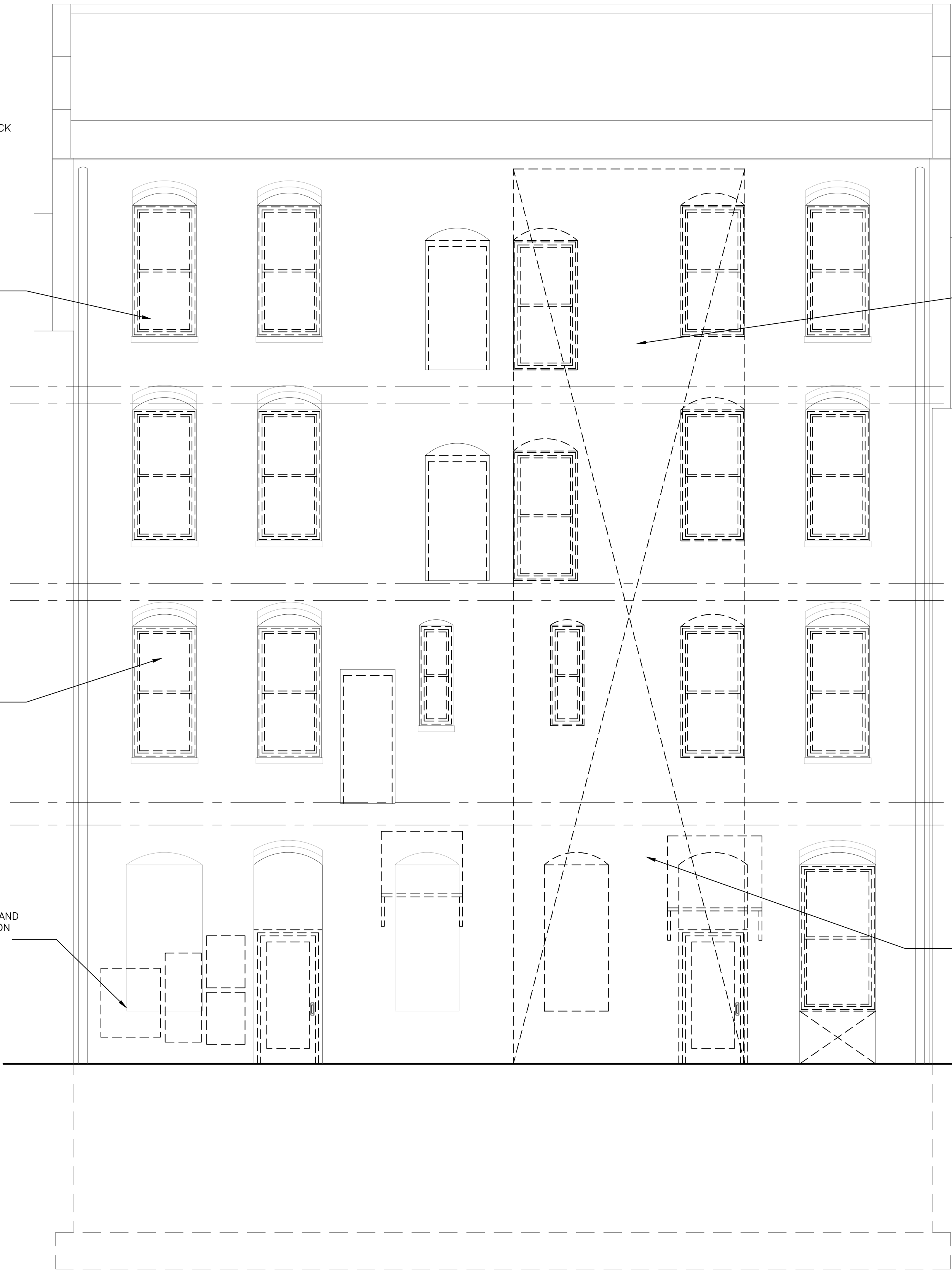
02 SOUTH DEMO ELEVATION SCALE: 1/4" = 1'-0"
