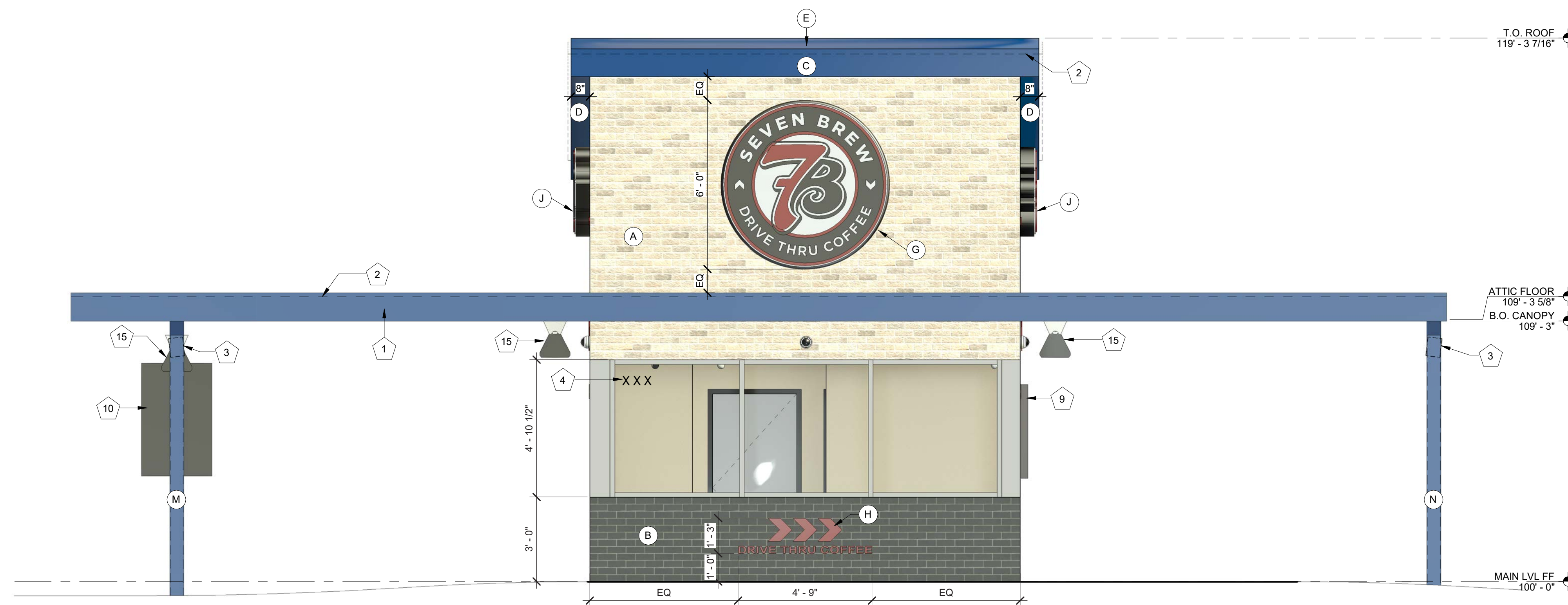
1 EXTERIOR ELEVATION - FRONT 3/8" = 1'-0"
