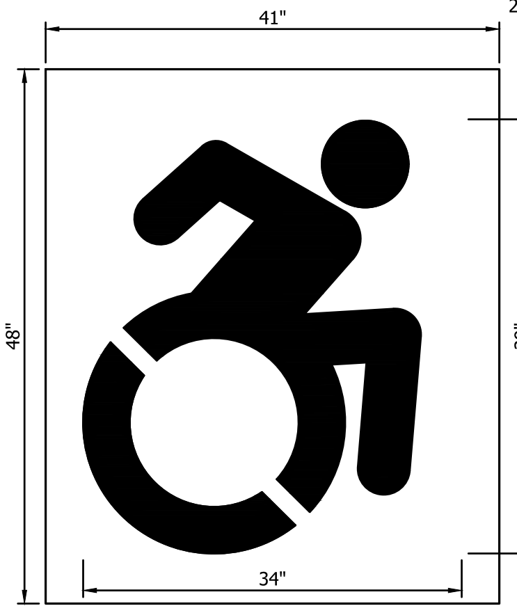
PAVEMENT MARKING (NOT TO SCALE)
