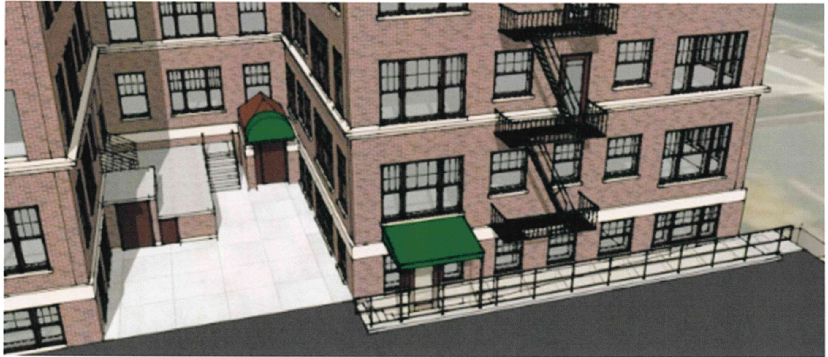
PRELIMINARY RENDERING OF PROPOSED EXTERIOR RAMP (CANOPY NOT PART OF FINAL DESIGN)
